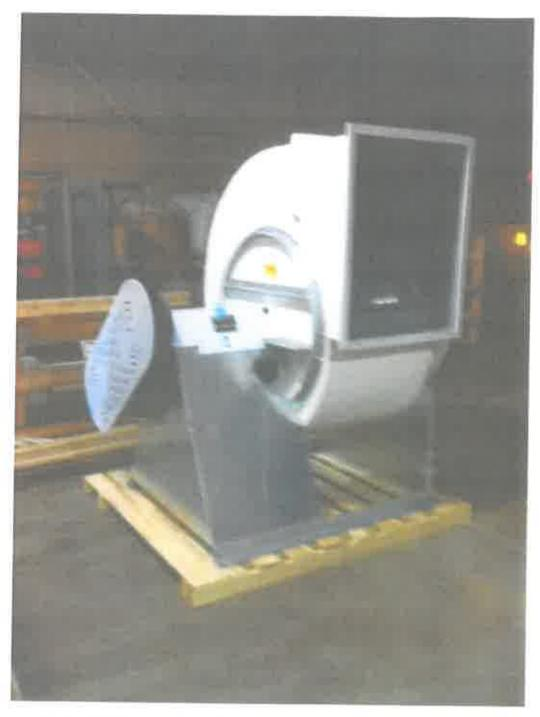
Typical NH Series Centrifugal DUALLast® FRP Exhaust Fan
